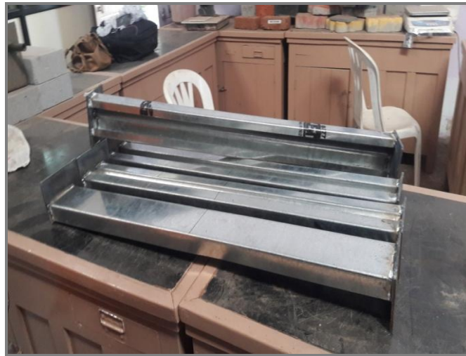
Fig 3 Specimens of cold formed steel channel section for the experimental work
