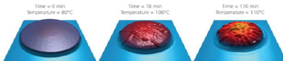
Figure 9: Annealing of shape memory polymer – Tapping mode topography images of a polystyrene (PS) microparticle during annealing. Scan size 12\ \mu\text{m} , Z (height) scale 1.4\ \mu\text{m} . The PS particle was flattened with a high-temperature, high-pressure nanoimprint lithography (NIL) process and then thinly coated with gold. Imaging began with the particle heated to 80^\circ\text{C} . The heater temperature was rapidly increased to 102^\circ\text{C} and then increased stepwise, so that it was 106^\circ\text{C} after 78 min, and 110^\circ\text{C} at 170 min. During annealing the particle diameter decreases and the height increases, recovering the original, pre-NIL spherical shape. A surface wrinkling morphology develops that gives information on recovery dynamics and strain energy release. Applications for micro- and nanoscale polymer particles include drug delivery and electronic packaging; incorporating shape memory effects could lead to many more. Imaged with the MFP-3D AFM. Adapted from Ref. 31
