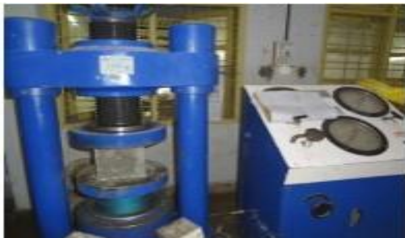
Fig. 2: Test specimen in compression testing machine.
