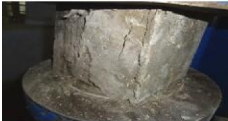
Fig. 3: Test specimen at failure
