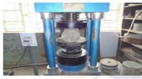
Figure 4: Concrete specimen in splitting testing Machine
