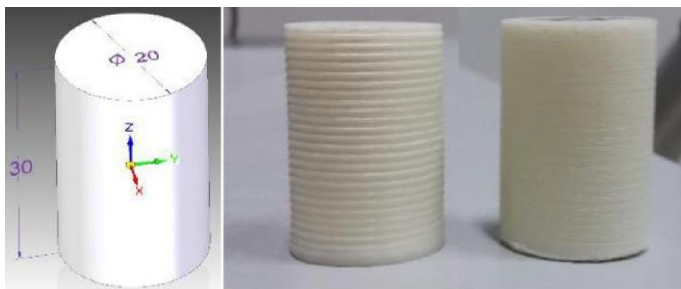
Fig.2. Dimensions of the analysed cylinder and two prototypes printed with 0.2mm (on the left) and 0.05 mm (on the right) layer thickness values
