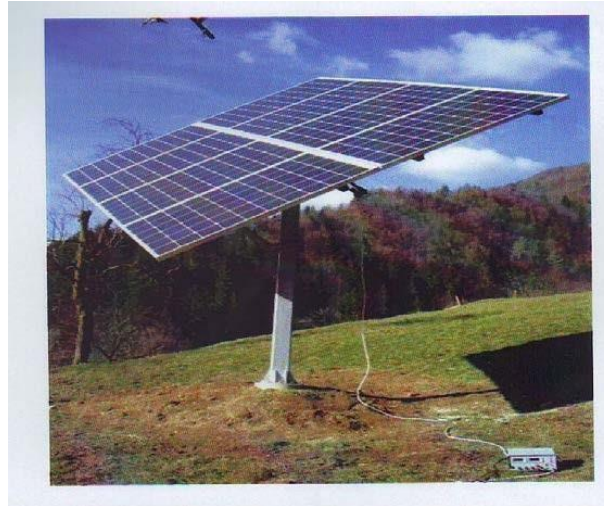
Fig. 3: Dual axis solar tracker
