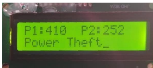
Figure 6. LCD Display at Electricity Theft Condition
