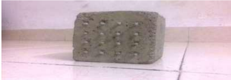
Figure 2: Light Transmitting Concrete Block.
