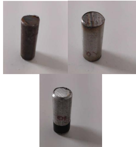
Fig 5. Sample Specimen of Grey Cast Iron, Stainless Steel
