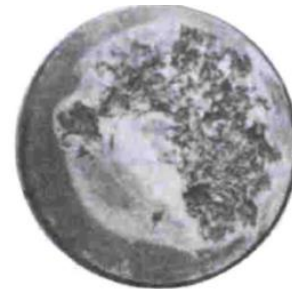
Fig 3.Pitting of Surface under Wear
