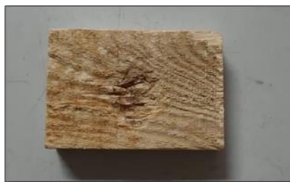
Figure 9. Damage for Deodar Fibre
