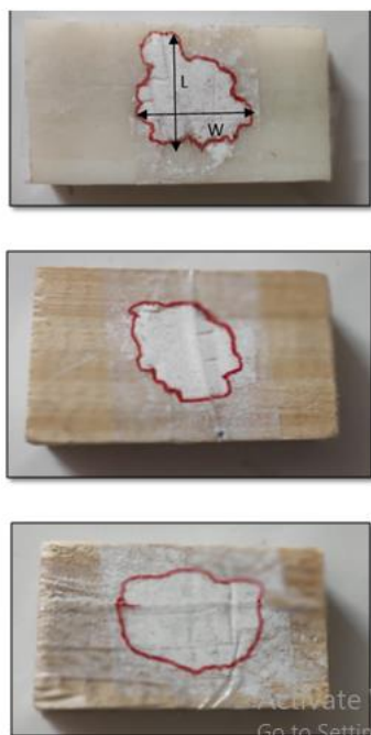
Figure 11. Procedure of Dye Penetrant Testing
