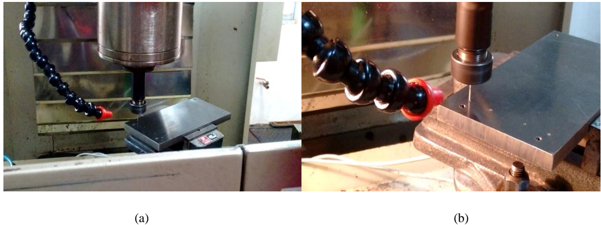
Fig 5 (a) Workpiece mounted on CNC Vertical Milling Machine (b) Drilling operation running
