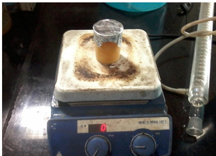
Fig 6 Preparation of nanofluid using magnetic stirrer
