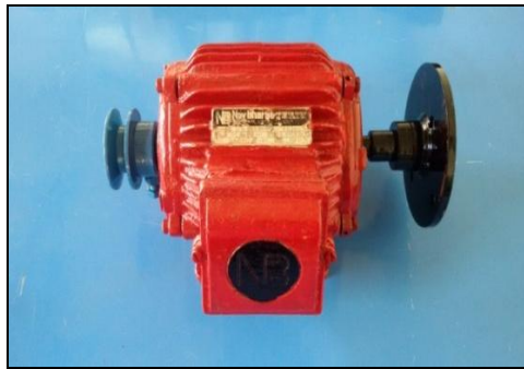
Fig. III. Motor with pulley and crank
