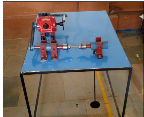
Fig. II. Fabricated model of combined fatigue testing machine
