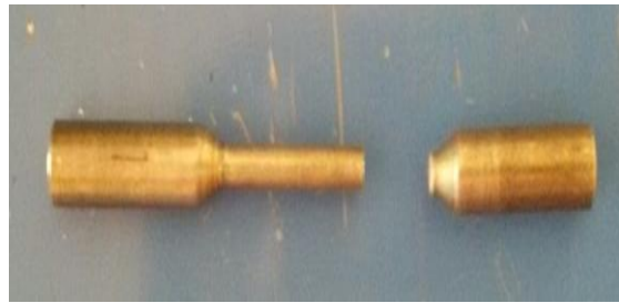
Fig. IX. 2. Rotating shaft fatigue testing specimen after failure
