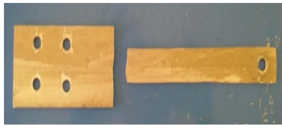
Fig. X. 2. Bending fatigue testing machine specimen after failure
