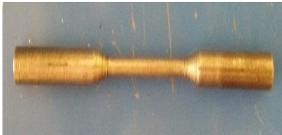
Fig. IX. 1. Rotating shaft fatigue testing specimen before failure
