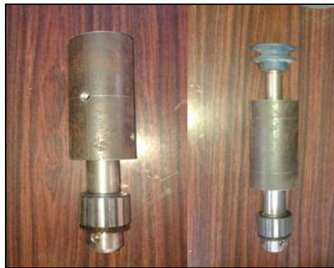
Fig. V. Assembly of shaft, bearings and drill chuck
