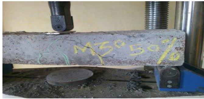
Fig.4 Flexural strength of beam.
