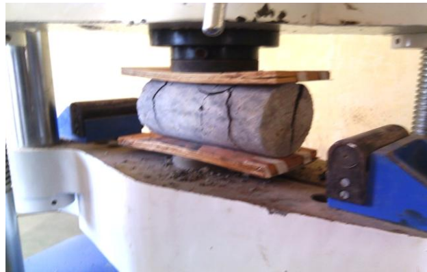
Fig. 3 Split Tensile strength test for cylinder
