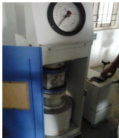
Fig 1: Testing of cube specimen using Compression Testing Machine
