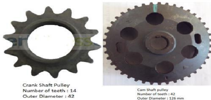
Figure 2 Timing Pulley For Six Stroke Engine
