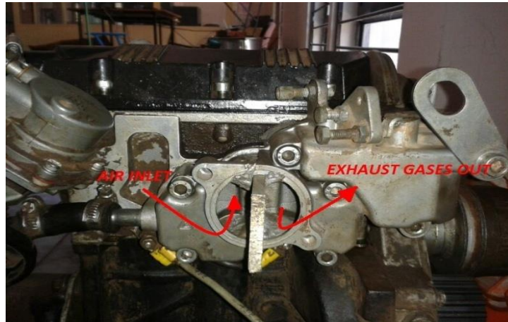
Figure 4 Modified Inlet and Exhaust Manifold of Six Stroke Engine
