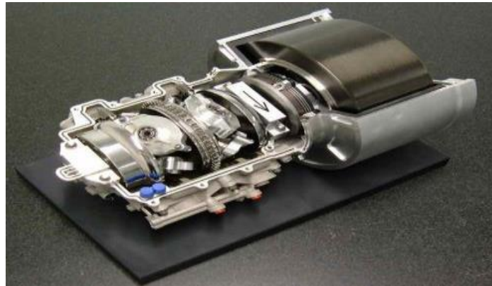
Figure 1: Flywheel for Kinetic energy recovery system of vehicle
