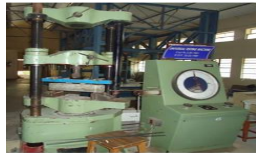
Fig 3 Flexural strength Testing using UTM
