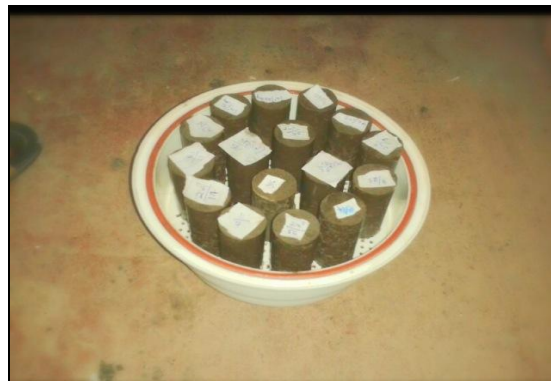
Fig 3.7.4.1 U.C.S. test samples in desiccator
