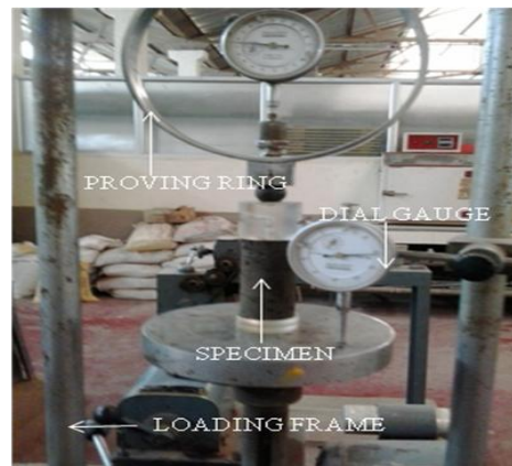
Fig.3.7.4.2 Unconfined compression test setup
