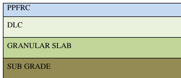
Figure4: Cross section of a typical PPFRC pavement
