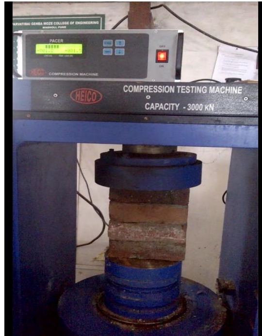
Fig: Model A1 (without binding wire, before failure) [Source- college Lab]
