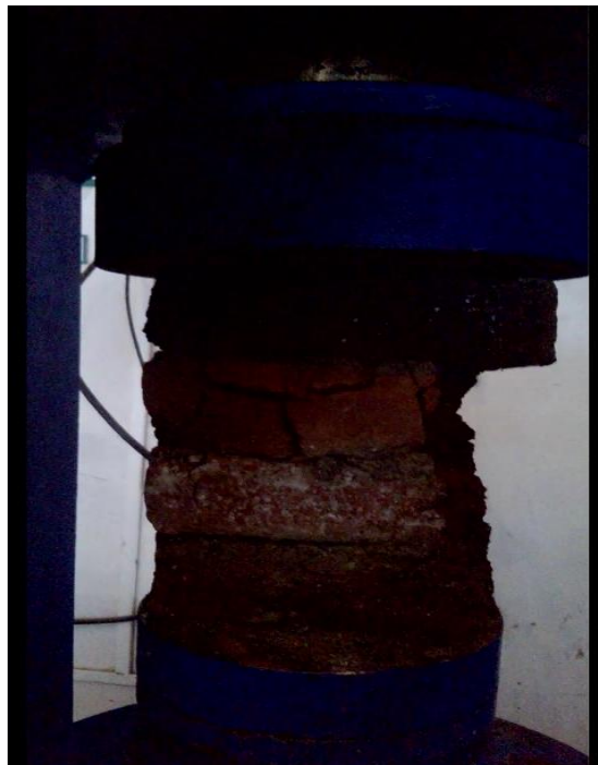
Fig: Model A1 (without binding wire, after failure) [Source- college Lab]
