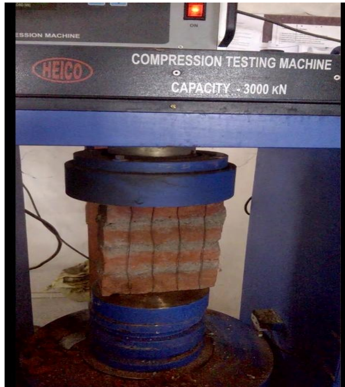
Fig: Model A2 (with binding wire, before failure) [Source- college Lab]
