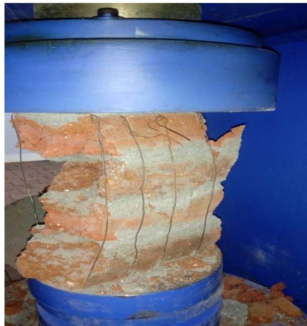
Fig: Model A2 (with binding wire, after failure) [Source- college Lab]
