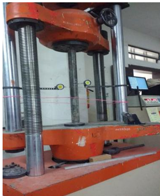
Fig.3 Test set up for CFST testing
