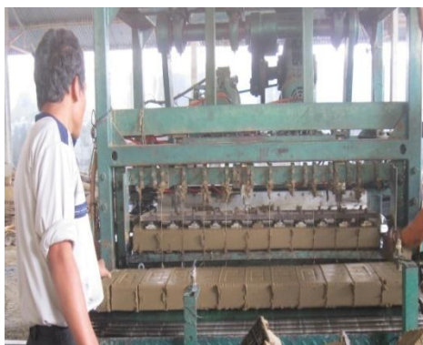
Figure:1- Manufacturing process of Mechanized bricks and Manual Bricks
