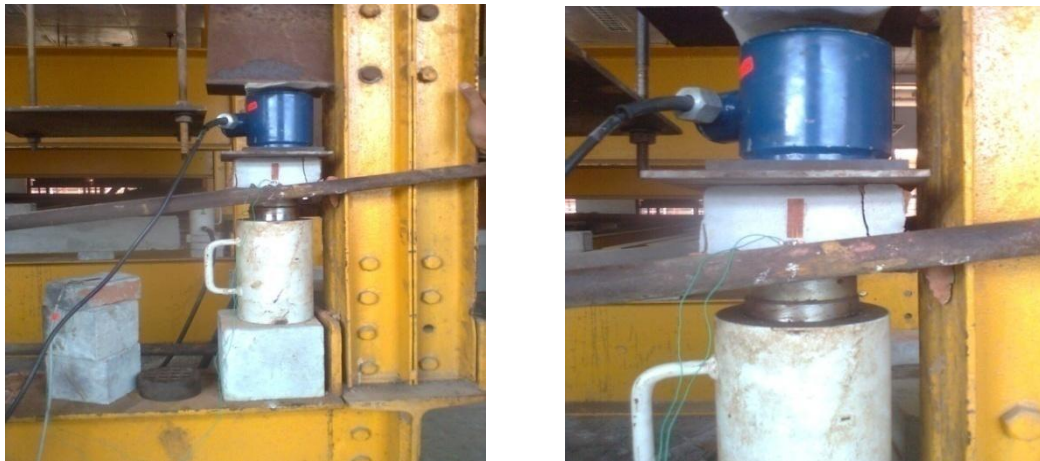
Figure:2- Experimental setup for strain measurement of clay brick.
