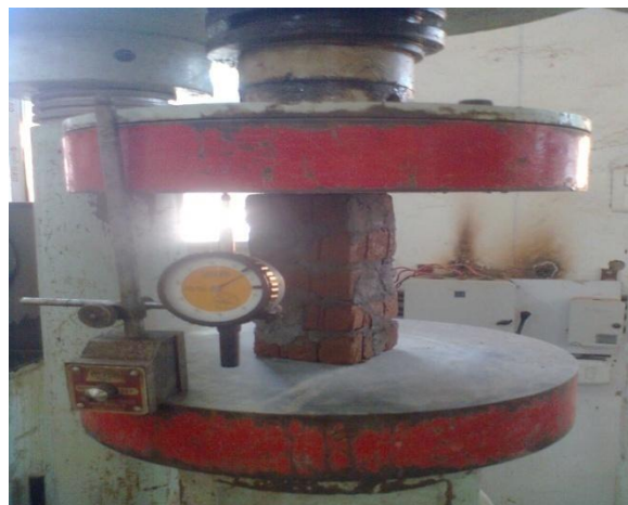
Figure:3- Experimental setup to find Elastic Modulus of Brick Prism
