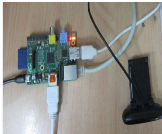
Fig 4 . Connection of USB Camera With Raspberry Pi
