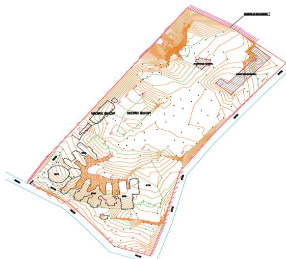
Figure 3:-Layout of Plane table & contour survey
