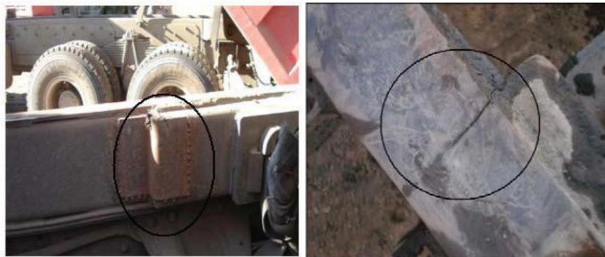
Fig.3.1.1 Fatigue crack of the sub-frame
