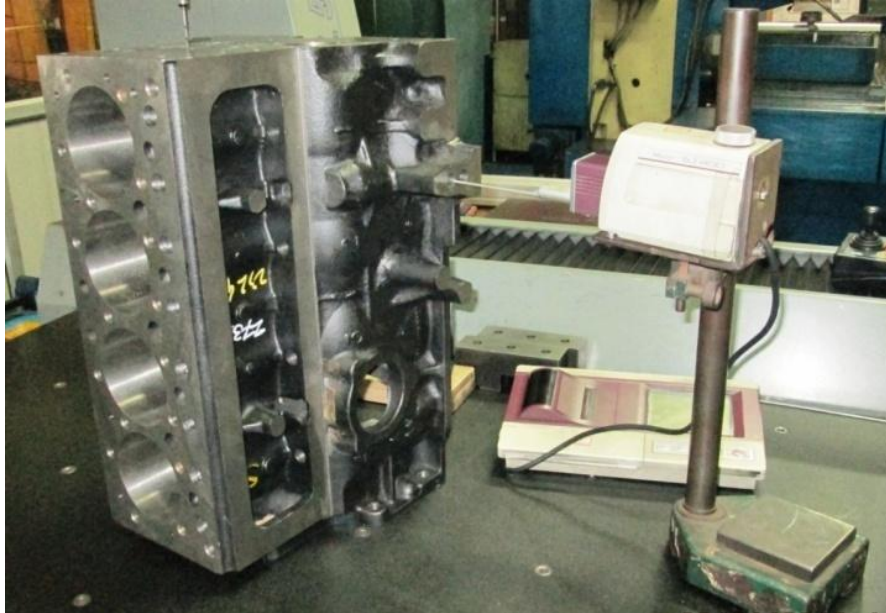
Fig. 2 Set up for measuring surface roughness
