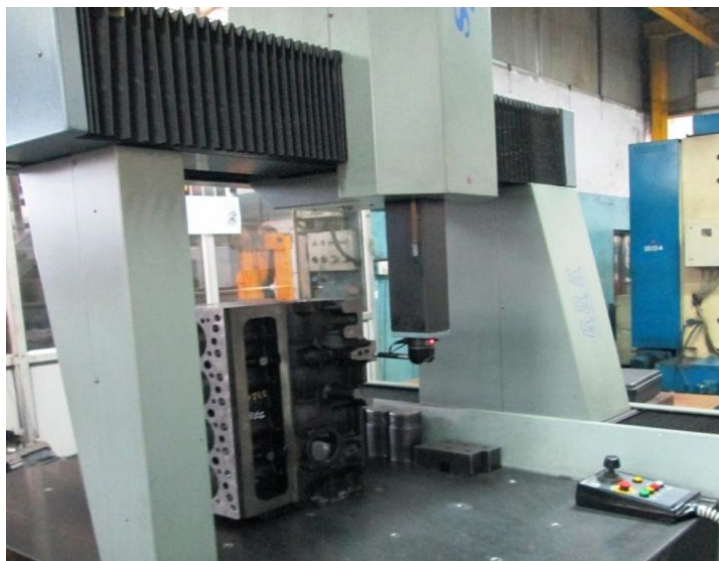
Fig.1 set up for measuring hole diametral error
