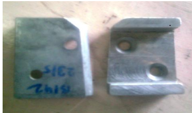
Figure 6. Finished product for Micro hardness and Surface roughness [After machining Dovetail]
