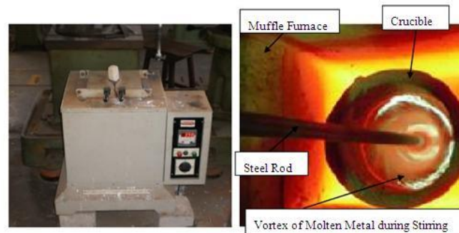
Figure 4. Muffle furnace and Preparation of samples
