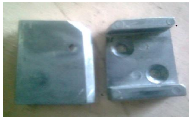
Figure 5. Synthesis of Al alloy with SiC composite using Stir casting route [As cast Dovetail]
