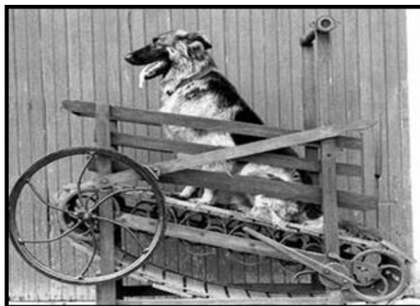
Fig 2. Dog Power Treadmill
