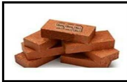
Photograph 2.1.1 Burnt Red Bricks
