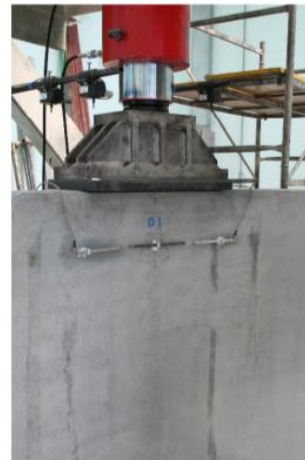
Fig.3 Point load test set up
