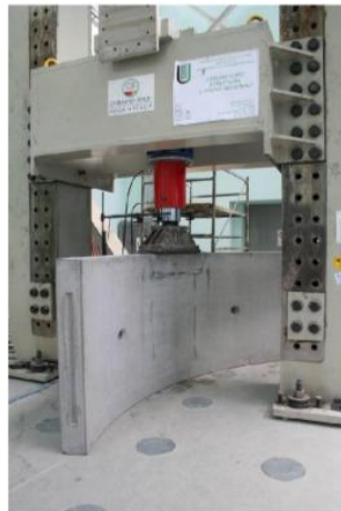
Point load test set up
