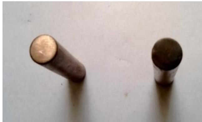
Fig. 1. Copper electrode used for machining.
