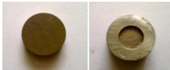
Fig. 2. AISI L2 steel sample before and after machining.
