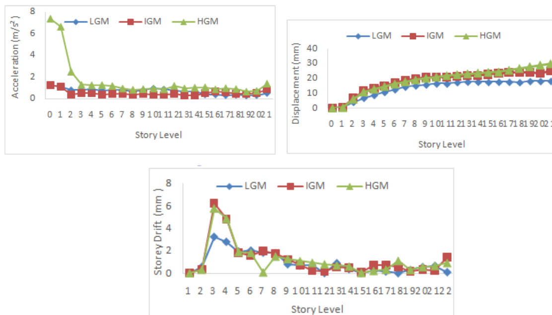
Figure 5(b): Floor acceleration, Floor displacement and Storey drift of twenty storeys RC building due to LGM, IGM and HGM in transverse direction
