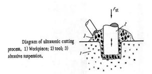
The working process of an ultrasonic machine is performed when its tool interacts with the workpiece or the medium to be treated. The tool is subjected to vibration in a specific direction, frequency and intensity. The vibration is produced by a transducer and is transmitted to the tool using a vibration system, often with a change in direction and amplitude. The construction of the machine is dependent on the process being performed by its tool.
