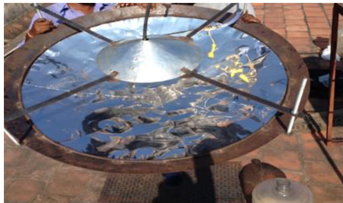
Fig.2 Photographic view of Schematic of Parabolic dish with conical coil setup
