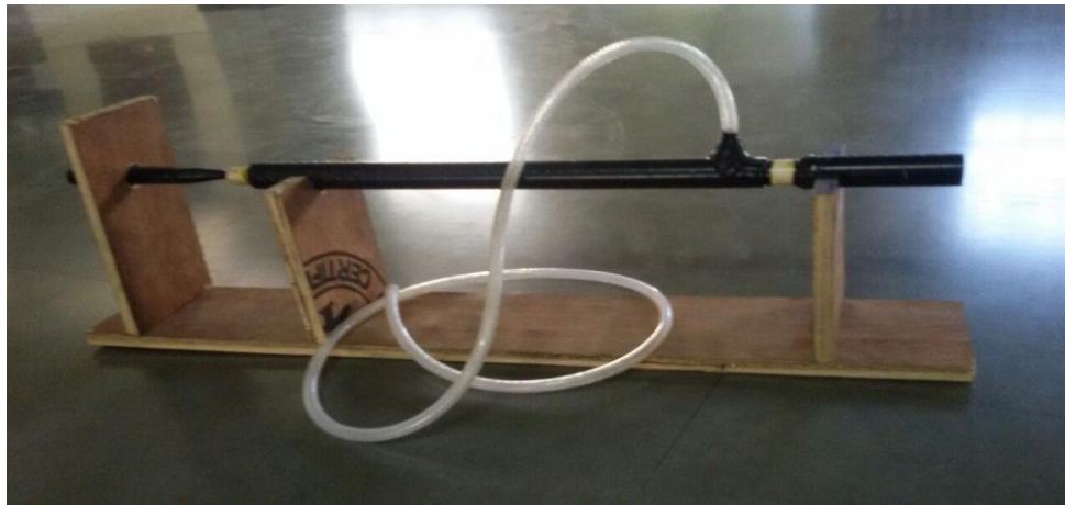
Fig 8. Fabricated Vortex Tube
