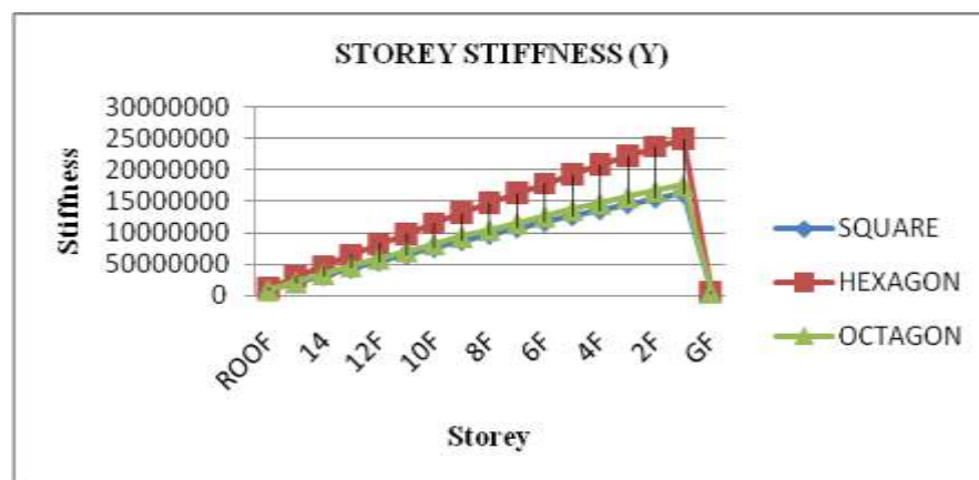
Fig.5.10 Storey Stiffness (Y)
