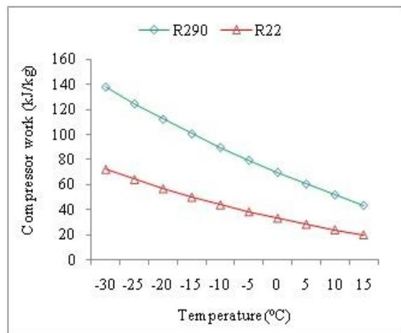
Figure 13: Compressor work Vs Temperature
