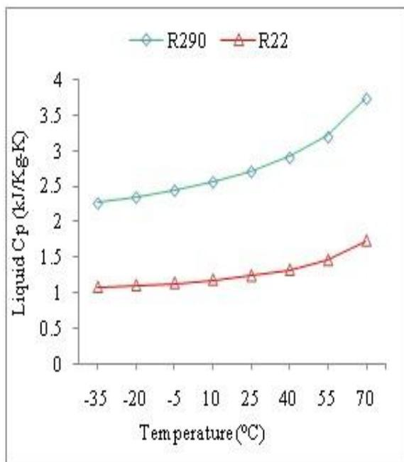
Figure 1: Temperature vs Liquid Cp.
