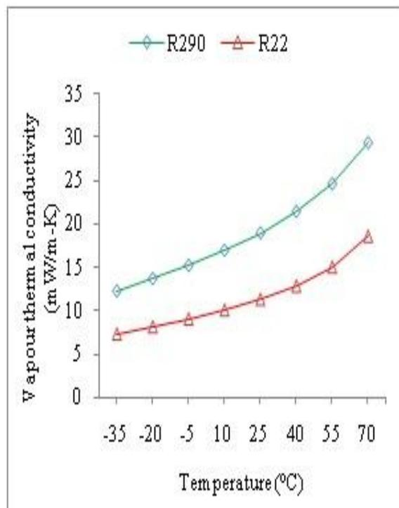
Figure 4: Temp. vs Vapour Thermal conductivity.
