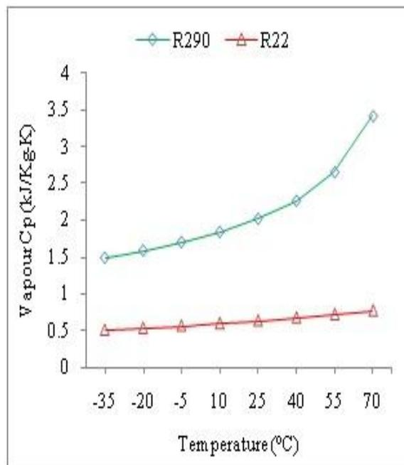
Figure 2: Temperature vs Vapour Cp.
