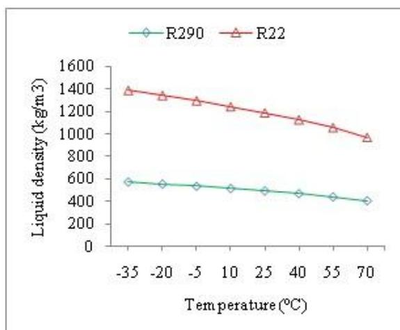
Figure 7: Temperature vs Liquid Density.
