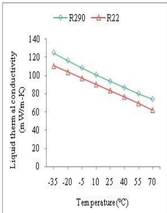
Figure 3: Temp. vs Liquid Thermal conductivity.
