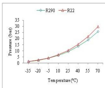
Figure 9: Temperature vs Saturation Pressure
