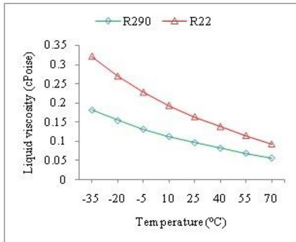
Figure 5: Temperature vs Liquid Viscosity.
