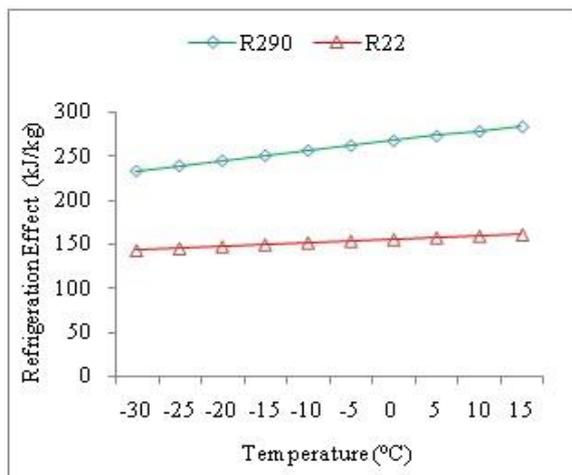
Figure 12: Refrigerating effect Vs Temperature
