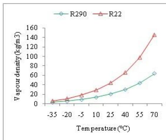
Figure 8: Temperature vs Vapour Density.
