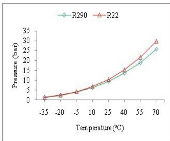
Figure 10: Pressure ratio Vs Temperature
