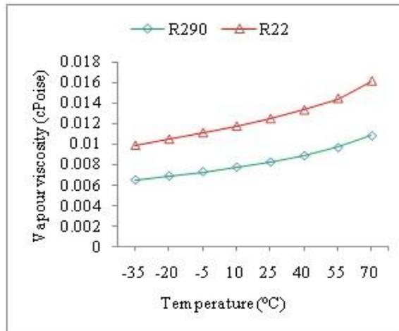
Figure 6: Temperature vs Vapour Viscosity.
