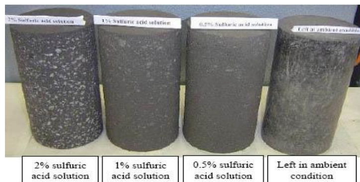
Figure No.3.1: Visual Appearance of Heat-cured Specimens after One Year of Exposure (Wallah and Rangan, 2006)
